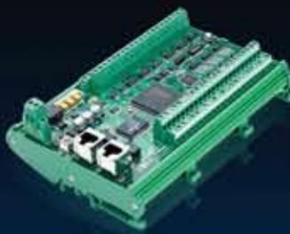
The **ZMP-SynqNet Series PC-based controllers** provide machine builders with the ultimate in highperformance motion control. The 64-bit ZMP controllers utilize a 466MHz PowerPC processor for optimum flexibility and speed. With a significant increase in processing power, the ZMP family of controllers are available in PCI and CPCI-3U form factors.
